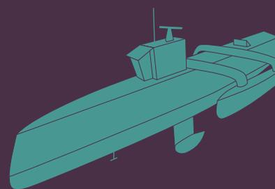
This 40m long self-navigating warship is designed to hunt for enemy submarines and can operate without contact with a human operator for 2-3 months at a time. It is currently unarmed. US representatives have said the goal is to arm the Sea Hunters and to build unmanned flotillas within a few years. However, it has been said any decision to use offensive lethal force would be made by humans.
