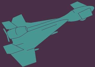
This 2.1m long 'loitering' missile is launched from a ground vehicle. It is armed with a 15 kg explosive warhead. The Harpy can loiter for up to 9 hours at a time, searching for enemy radar signals. It automatically detects, attacks and destroys enemy radar emitters by flying into the target and detonating.
